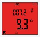
If the difference exceeds the programmed threshold, the **×** symbol is displayed and the backlight turns red.
