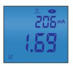
PI Test Time Measurement Default measurements are at 1 minute and 10 minutes
